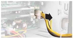
4 Pull the power supply release lever out (toward you) until the power supply slides freely, then slide the power supply out of the computer.
